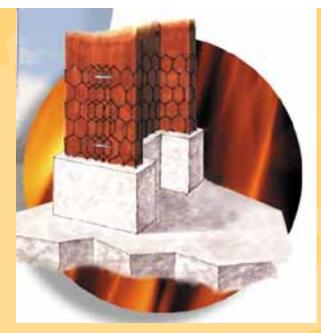
3.3 cementitious mixtures: As defined by UL in "Spray Applied Fire Resistive Materials" (SFRM), cementitious mixtures are binders, aggregates and fibers mixed with water to form a slurry conveyed through a hose to a nozzle where compressed air sprays a coating; the term is sometimes used for materials (such as sand and cement) applied by either spray or trowel.
